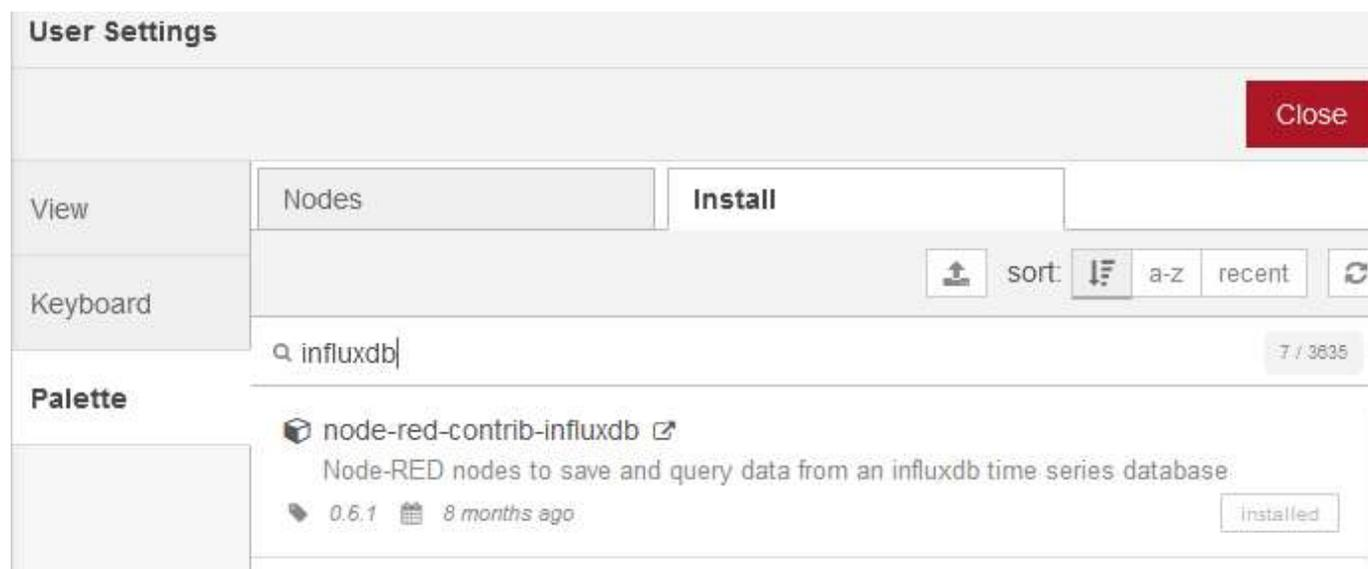
The screenshot shows the 'User Settings' dialog box in Node-RED. The 'Nodes' tab is selected, and the search bar contains 'influxdb'. The search results show a node named 'node-red-contrib-influxdb' with a description: 'Node-RED nodes to save and query data from an influxdb time series database'. The version is '0.6.1' and it was updated '8 months ago'. An 'installed' button is visible next to the node name.
